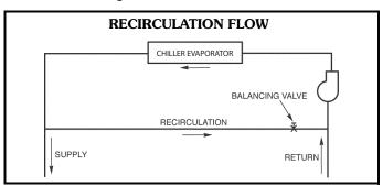
The maximum evaporator flow (approximately  $5\,^\circ$  F (2.8  $^\circ$  C) rise results in a practical maximum pressure drop through the evaporator. Optional marine waterboxes may help reduce pressure drop by a small amount. If this is insufficient, a return fluid may bypass the evaporator to keep the pressure drop through the evaporator within acceptable limits. This permits a higher delta T with lower fluid flow through the evaporator and mixing after the evaporator.
